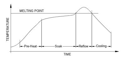
Lead-free solder (SnCuAg) is a viable alternative to leaded solder that significantly reduces health concerns and environmental impact. Lead-free solder typically has a high tin concentration, making this the most expensive option. In addition, tin has a higher melting point with a thermal profile of 150°C /190°C /250°C . Lead-free solder works well if the design and components can withstand higher heat exposure.
